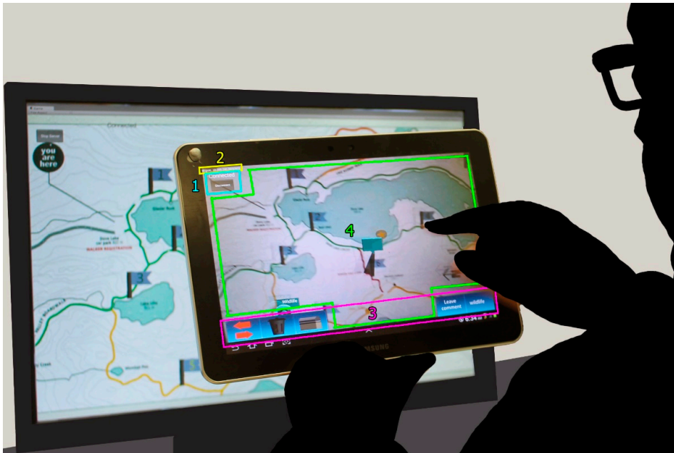
Figure 3. User Interface, showing the server connection button (1); log information (2); input buttons (3); and the input area (4).
