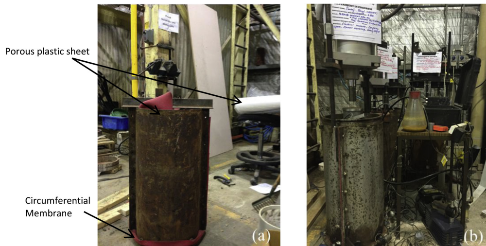
Fig. 5. (a) Installation of membrane around the undisturbed specimen for vacuum case (US3), and (b) Final setup of sample for vacuum case.
