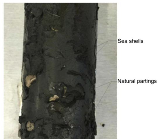
Fig. 9. Soil sample showing the presence of large shells and natural partings.
