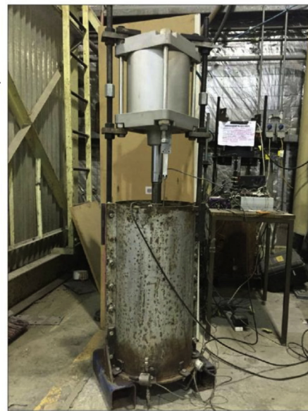
Fig. 3. Large-scale consolidometer with US1: (a) Schematic diagram, and (b) Laboratory setup.
