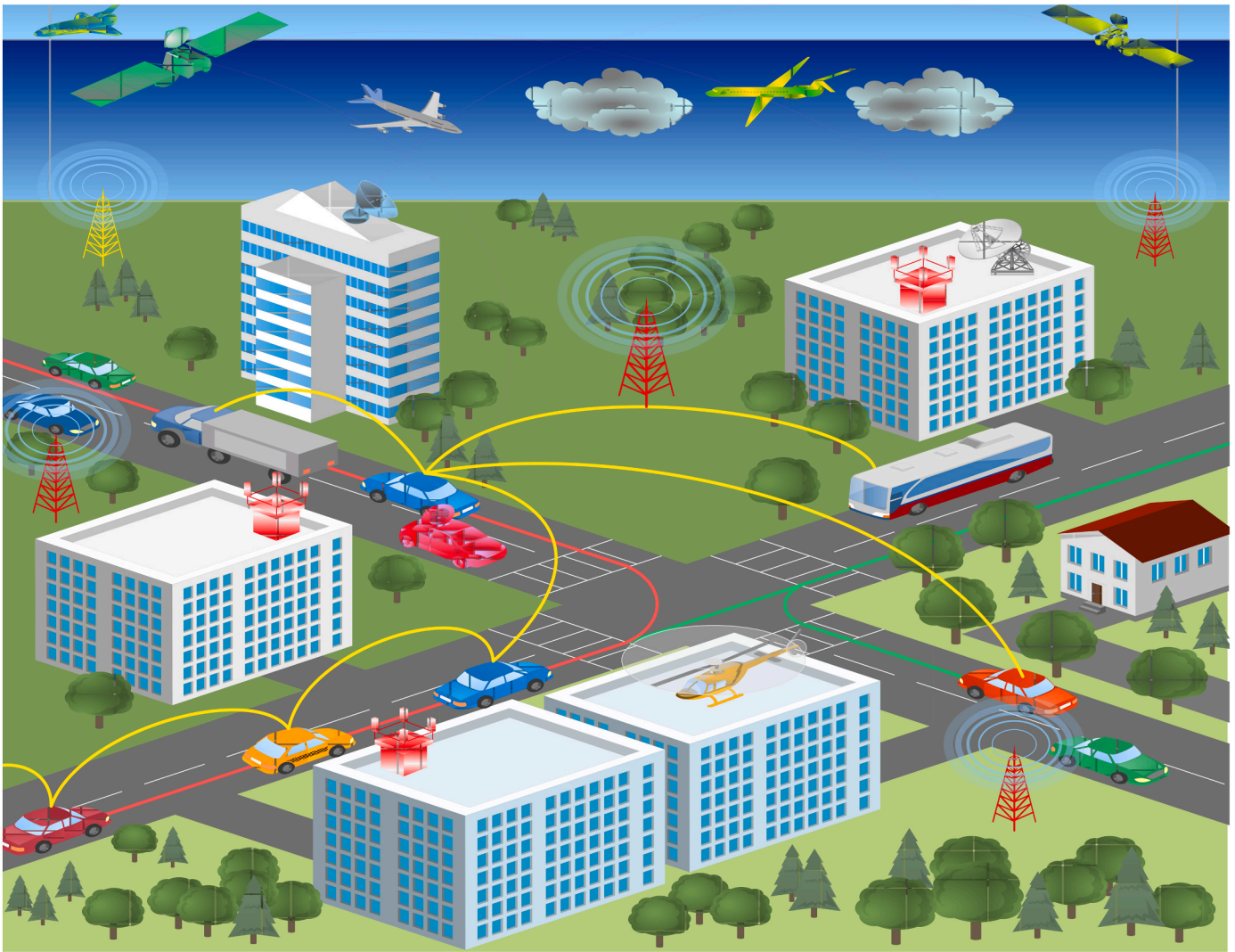
Fig. 17. Overview of Smart Transport Infrastructure showing the smart transport infrastructure communication theme. The purple communication lines are between communication providers within STI. Yellow colour lines represent the communication between the infrastructure participants, i.e., smart vehicles. An increase in traffic density requires increased bandwidth, and at the larger scale of city-level STI, satellite and high-speed communication can result in optimized operations of overall infrastructure. (For interpretation of the references to colour in this figure legend, the reader is referred to the web version of this article.)
