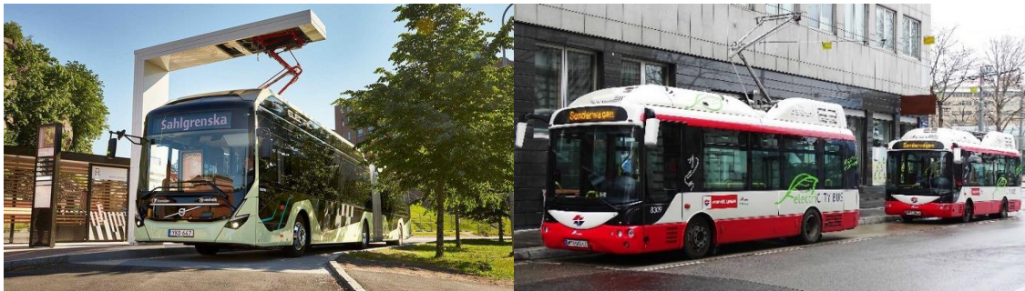
Figure 12 – (Left) Volvo bus with a rooftop pantograph for opportunity pantograph charging.
