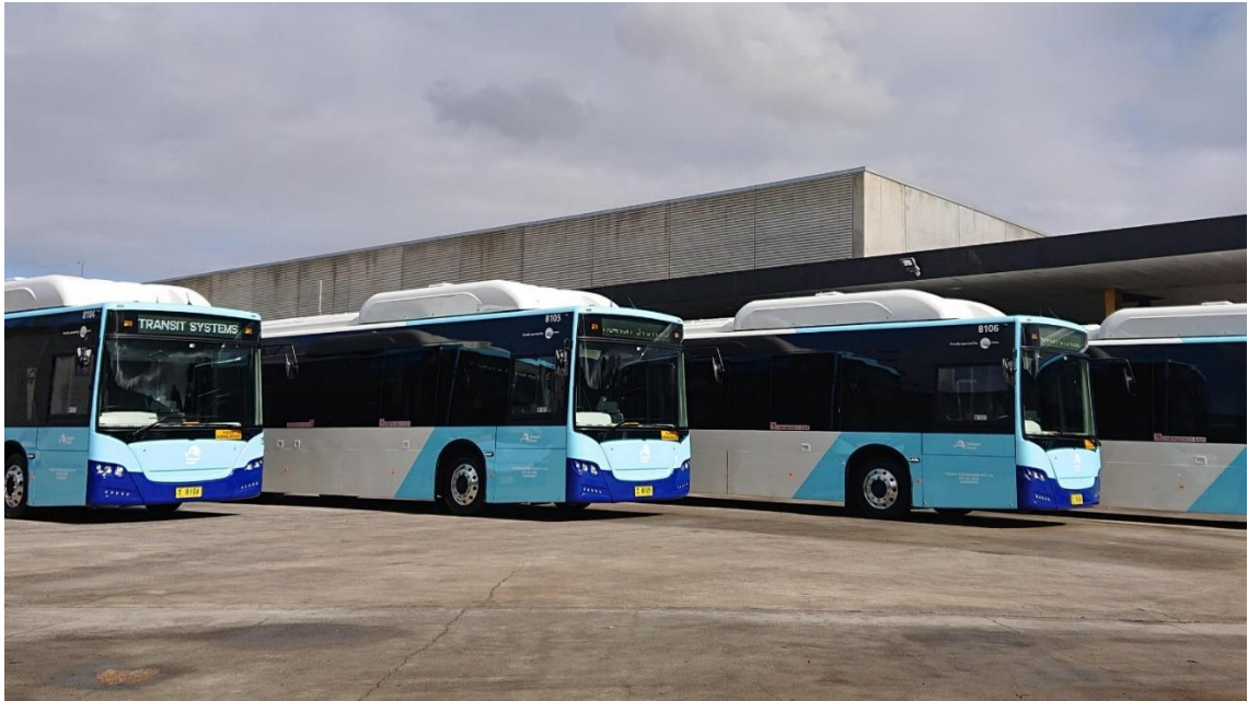
Figure A5 – BEV bus with BYD chassis and Gemilang body (Transit Systems 2019).
