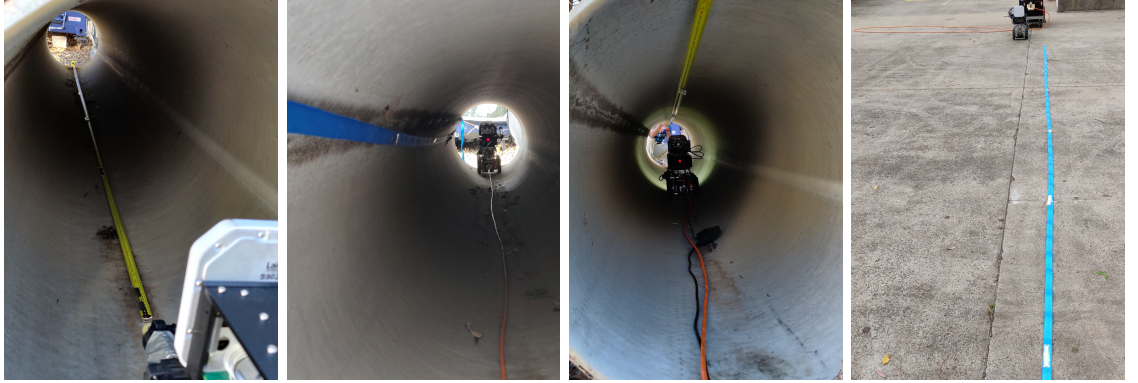
(b) RFID tags placed on the bottom of the pipe.
