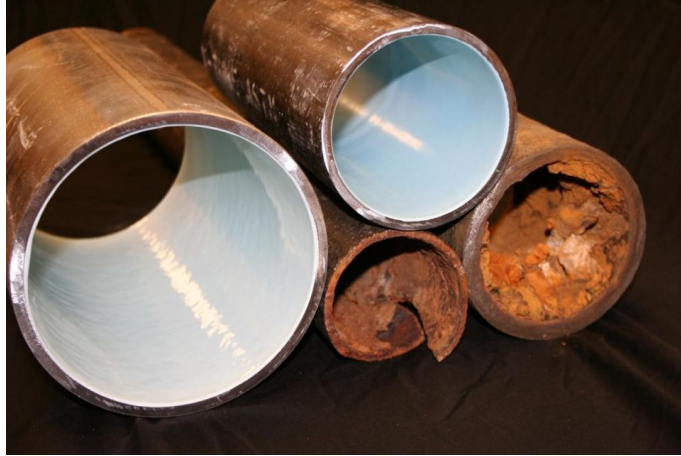
FIGURE 1.1: Corroded and liner applied pipe samples [1].
