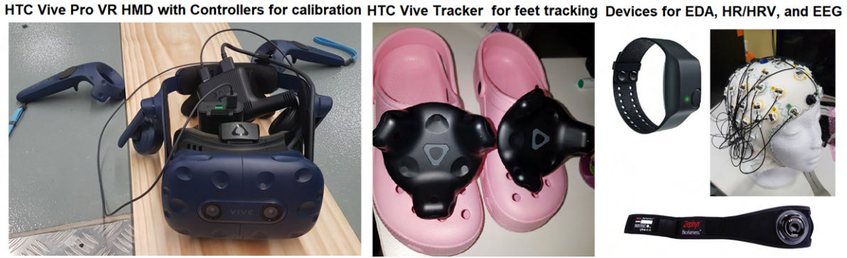
Figure 3.8: The equipment used in this experiment for VR visualisation, tracking, and physiological measurements.
