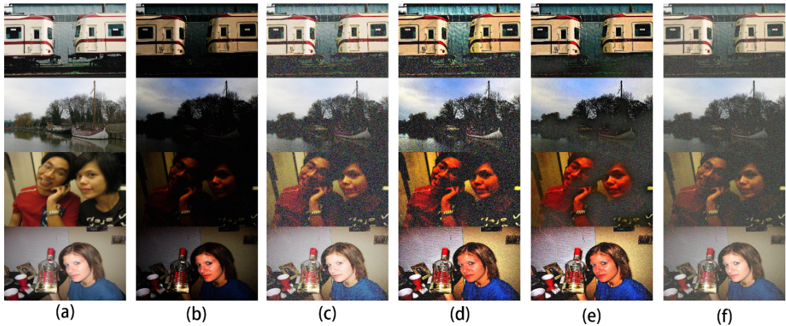
Figure 2.5 : Examples of image enhancement results obtained on the synthetic dataset with benchmark approaches and our proposed approach. (a) Ground truth. (b) low light images. (c) MSR [40] results. (d) LIME [28] results. (e) LECARM [126] results. (f) Our results.
