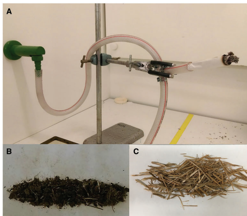
Figure 1: Generation of CDSE and WSE. (A) A water aspirator was set up to draw smoke from a burning cow dung or wood shaving roll using the vacuum created by the flow of water. (B) Cow dung was sun-dried, crushed into fine particles, and rolled in paper. (C) Wood was cut into small chips and rolled in paper.
