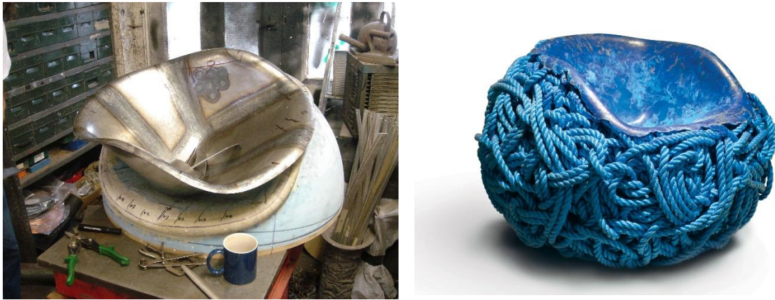
Fig. 8.11. Former based on Eames arm chair used to make impression for Tom Price's Meltdown Chair . Source: Tom Price
