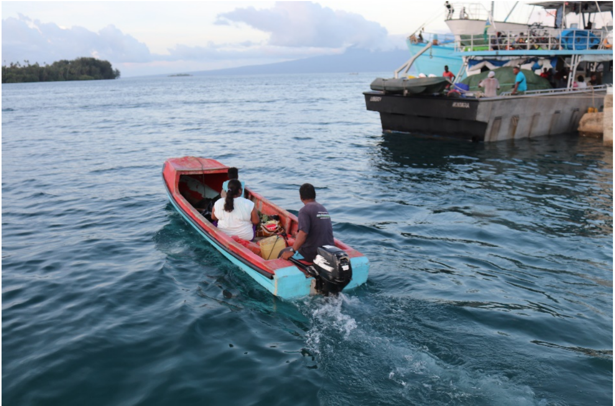
Figure 47. A typical vessel with a 15 hp engine used for handline tuna fishing in oceanic waters (Photo: Nick McClean).
