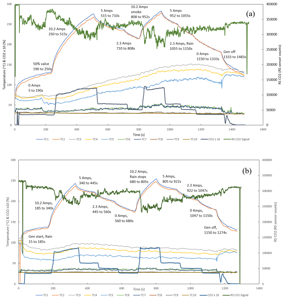
Figure 6.4: Resistor load bank test for revised calibration device.
