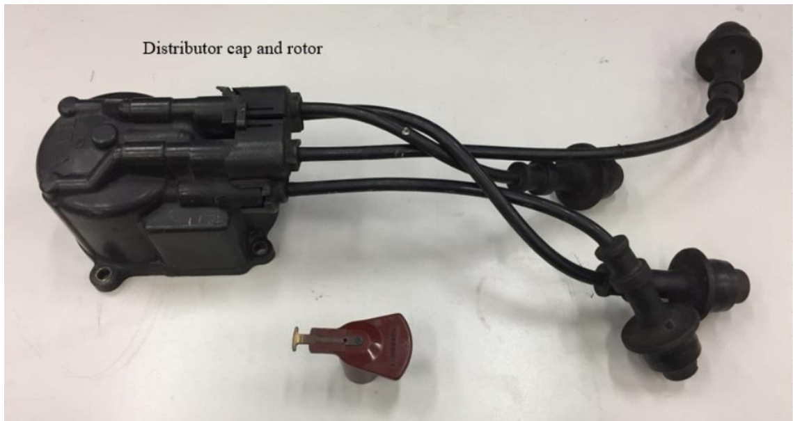
Figure 3.7: Worn Ignition system hardware for experimental testing.
