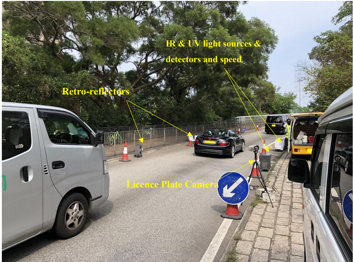
Figure 3.3: Setup of a typical RS measurement site in Hong Kong, China.
