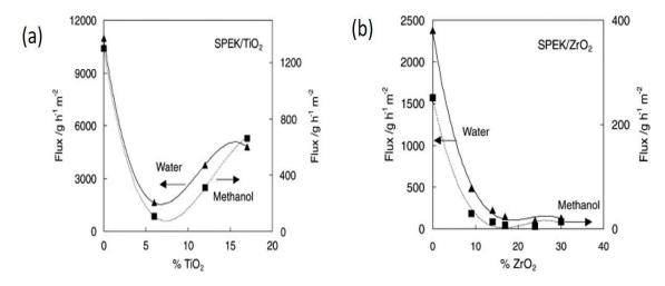
**Figure 6.** Methanol and water flux in pervaporation experiments at 55 °C post modification of a SPEK membrane with (a) TiO<sub>2</sub> and (b) ZrO<sub>2</sub>. Reprinted with permission from [72]. Copyright (2002) Elsevier Science B.V.
