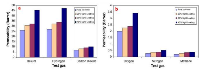
**Figure 8.** Comparison between gas permeability of pure Matrimid and its nanocomposite membranes having different concentrations of MgO NPs; (**a**) shows the comparison of helium, hydrogen, and carbon dioxide; (**b**) shows the comparison of oxygen, nitrogen, and methane. Reprinted with permission from [87]. Copyright (2007) Elsevier B.V.
