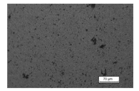
**Figure 4.** Differential coefficient interference pattern of Al<sub>2</sub>O<sub>3</sub>-particle distribution in the modified membrane. Reprinted with permission from [69]. Copyright (2006) Elsevier B.V.
