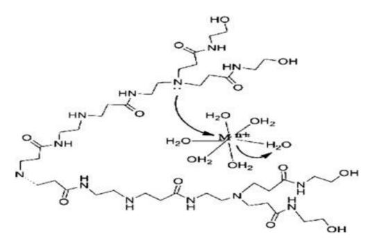
**Figure 2.** Mechanism for metal cations removal by PAMAM dendrimers–titania composites. Reprinted with permission from [12]. Copyright (2013) Elsevier Ltd.
