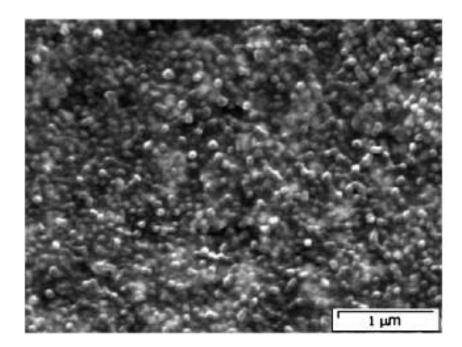
**Figure 7.** SEM of a SPEK membrane modified with 22 wt.% TiO<sub>2</sub>. Reprinted with permission from [72]. Copyright (2002) Elsevier Science B.V.
