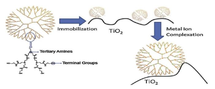
**Figure 1.** Strategy for immobilizing G4-OH dendrimers on titania to produce dendrimer/titania composites. Reprinted with permission from [12]. Copyright (2013) Elsevier Ltd.
