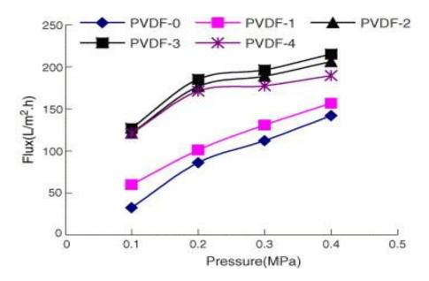
**Figure 3.** Distilled–H<sub>2</sub>O fluxes of membranes having different compositions of nano-sized Al<sub>2</sub>O<sub>3</sub> particles. Reprinted with permission from [69]. Copyright (2006) Elsevier B.V.
