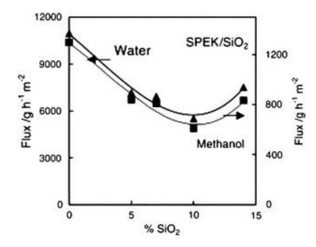
**Figure 5.** Methanol– $H_2O$  flux in pervaporation experiments at 55 °C by modification of an SPEK membrane with hydrolyzed TEOS. Reprinted with permission from [72]. Copyright (2002) Elsevier Science B.V.
