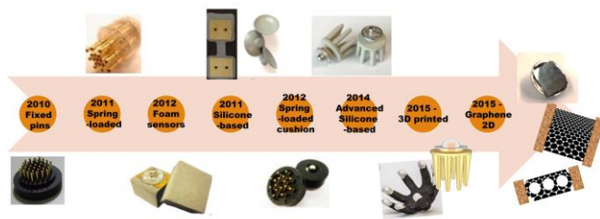
Fig.5 Recent evolution of dry EEG sensors. Acicular designs and advanced conductive materials and fabrication options have been investigated in recent years. Notably, graphene has more recently joined the class of investigated materials, holding promise of superior biocompatibility and electrical conductivity.
