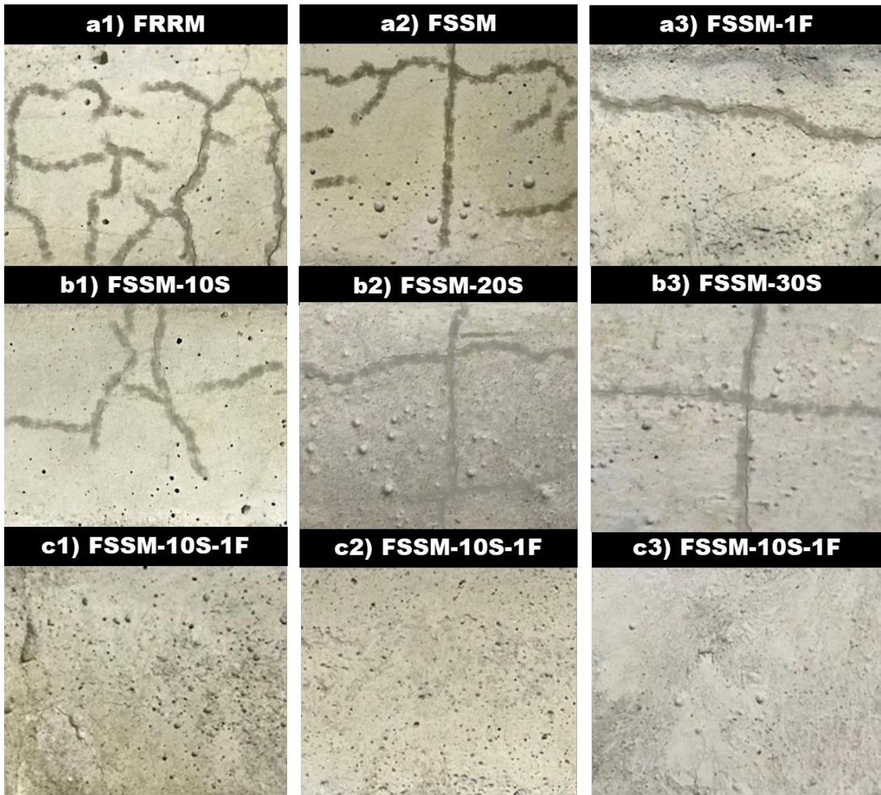
Figure 6.5. Visual appearance of all mortars after exposure to a temperature of 700 °C
