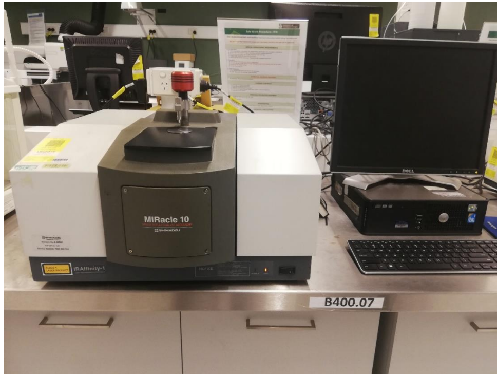
Figure 3.13 Photo-Image of Fourier transforms Infrared (FTIR)
