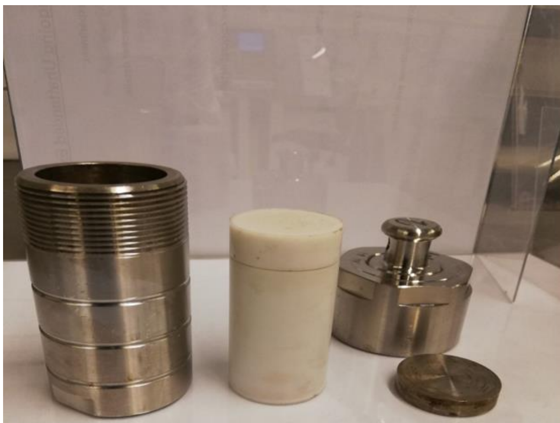
Figure 3.2 Image of the Teflon-lined vessel reactor used in this study
