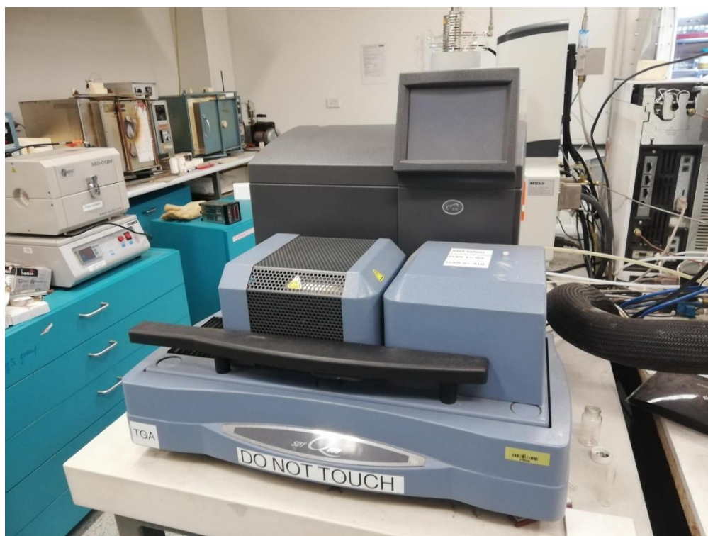
Figure 3.8 Photo-Image of the thermal gravimetric analysis (TGA)
