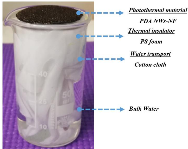
Figure 6.2 Photo-image of the designed PDA NWs driven solar evaporator.
