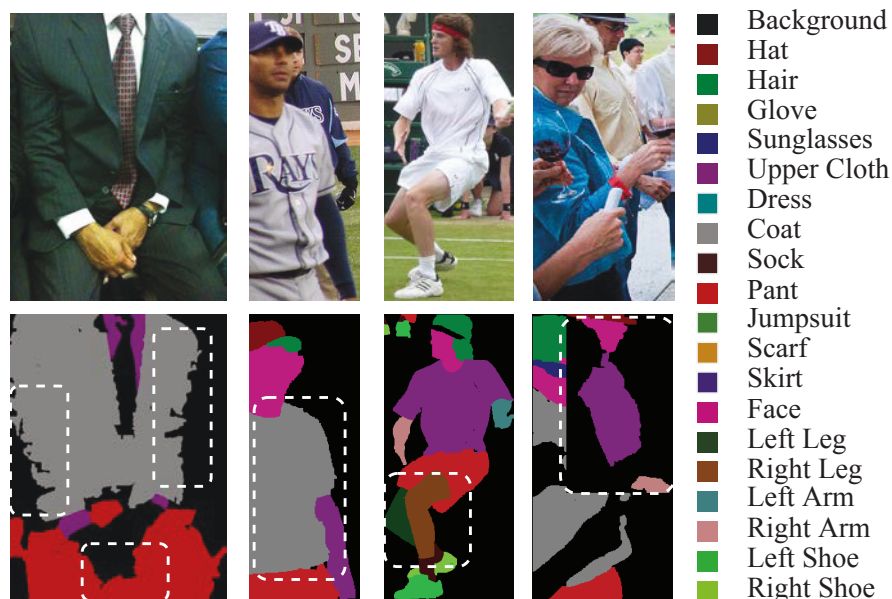
Figure 3.1: Different types of label noises in ground-truth annotations. The upper row shows the original images. The lower row shows the original ground-truth labels. Different types of noisy labels are illustrated from left to right, (a) coarse annotation around the boundary area; (b) confused fine-grained categories, where the upper-cloth is mislabeled as the coat; (c) confused mirror categories, where the right leg is mislabeled as the left leg; (d) multiple-person occlusion. Annotation noises are marked in white dashed boxes.
