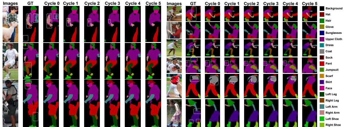
Figure 3.6: Examples from LIP train set during our self-correction process. Label noises like inaccurate boundary, confused fine-grained categories, confused mirror categories, multiple person occlusion are alleviated and resolved during the process. The boundaries of our corrected label are prone to be more smooth than the ground-truth label. Label noises are highlighted by white dotted boxes. Better zoom in to see the details.
