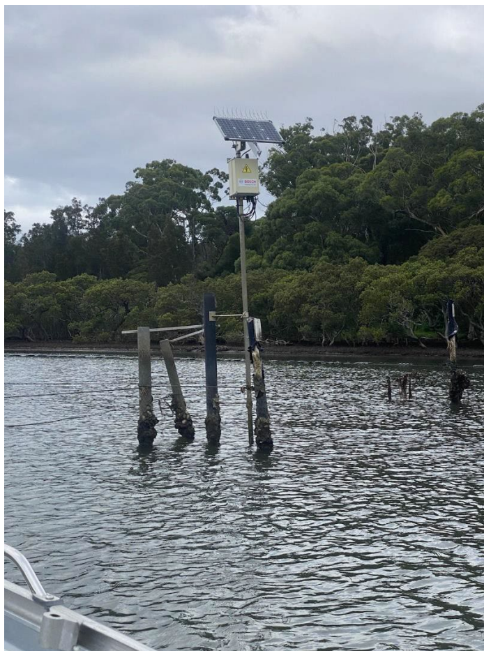
Figure A2 Seabird MicroCAT high accuracy conductivity, temperature and depth (CTD) field sensor deployed in the Shoalhaven and Crookhaven Rivers. Image supplied by Angela Riepsamen.
