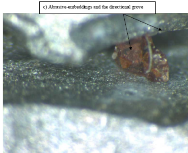
FIGURE 8: The patterns on an aluminium specimen eroded by a fast moving cavitating water jet submerged, with the common features of the directional grooves, and the abrasive embedding [x245].
