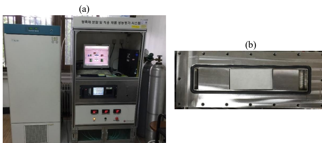
Fig. 3-4. Experimental setup for the UV-based photocatalysis of acetaldehyde (a), sample holder in the reactor (b).
