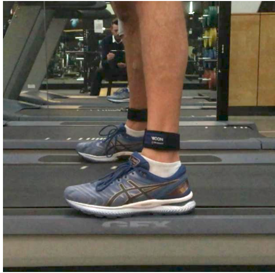
Figure 7.3: The placement of the IMU device on the ankle area of a participant.
