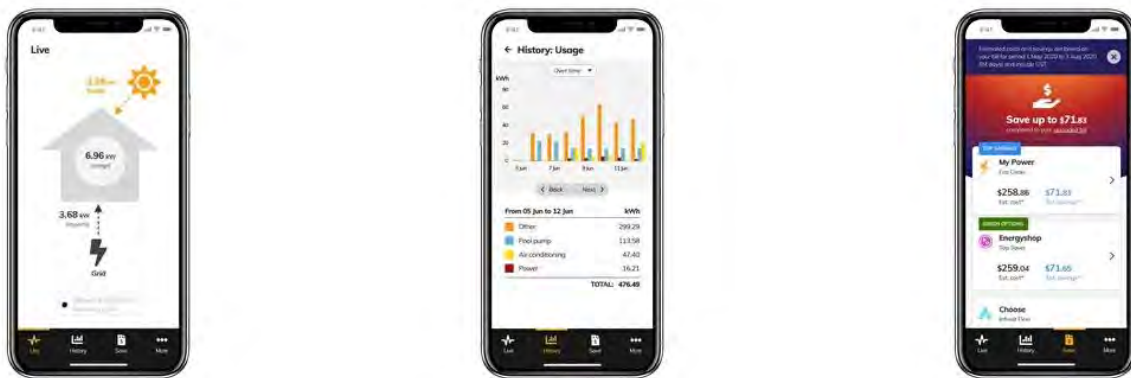
Figure 13 - MyData.Energy app examples of real time consumption (left), circuit level monitoring (middle) and energy plan comparison (right)
