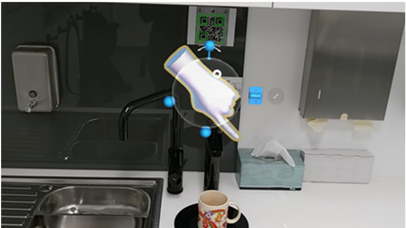
Figure 7. A symbol in the Guide installation environment with switches (blue dots and rectangle) to size and orient.
