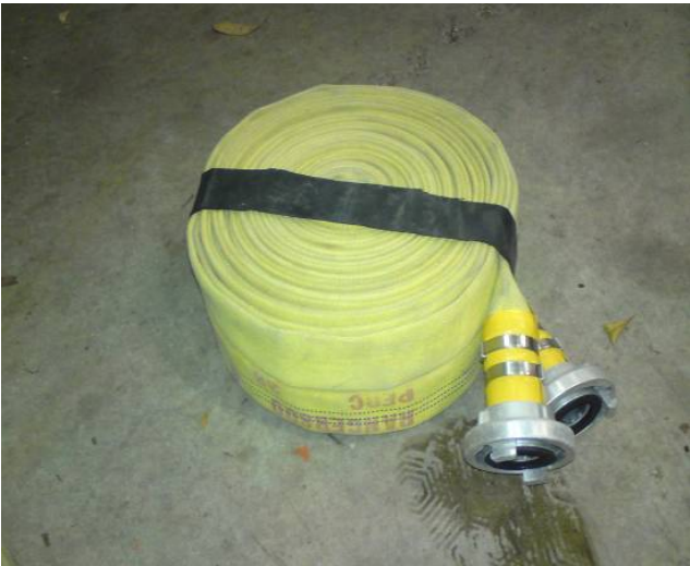
Figure 3. Percolating hose used to deliver water for fire-fighting.
