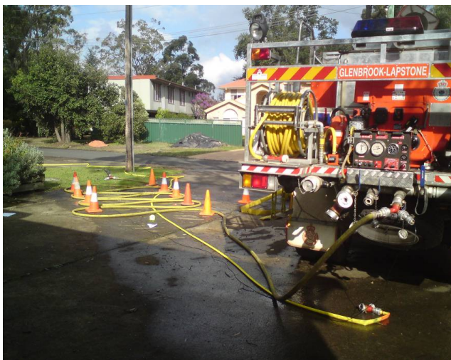
Figure 8. Photo of a test set-up with hose having severe bends.
