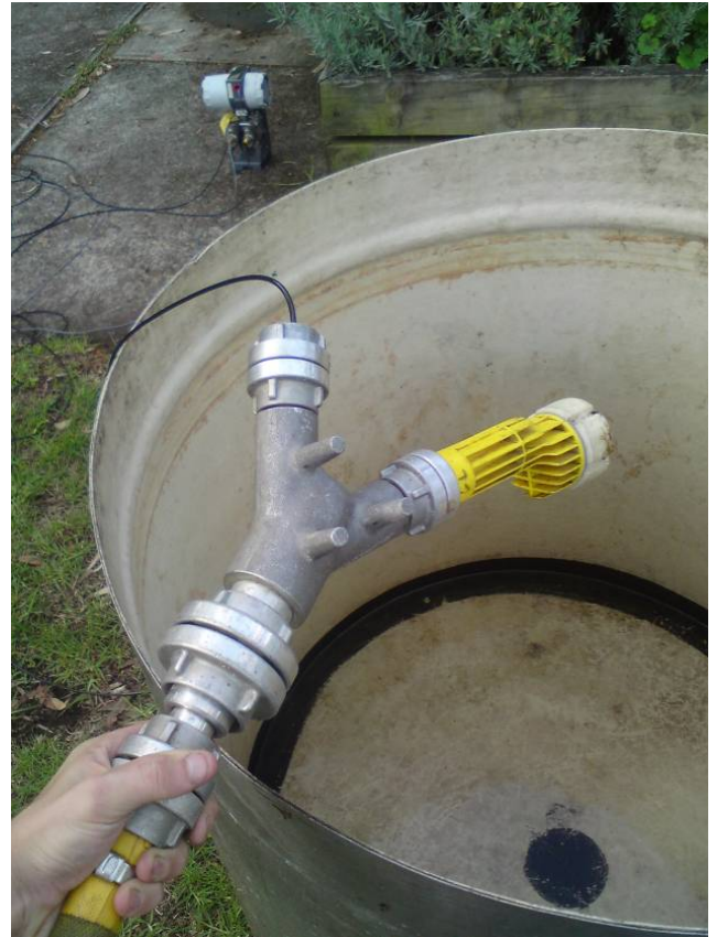
Figure 5. Photo of a nozzle with pressure line attached (for pressure P2 in figure 4) and the water drum.
