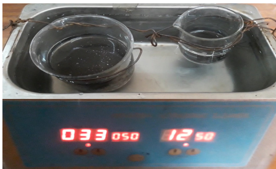
Figure 2. During the blends formation of synthetic lubricant, two beakers were kept into Sonicator Bath for 20 min at 50 °C.
