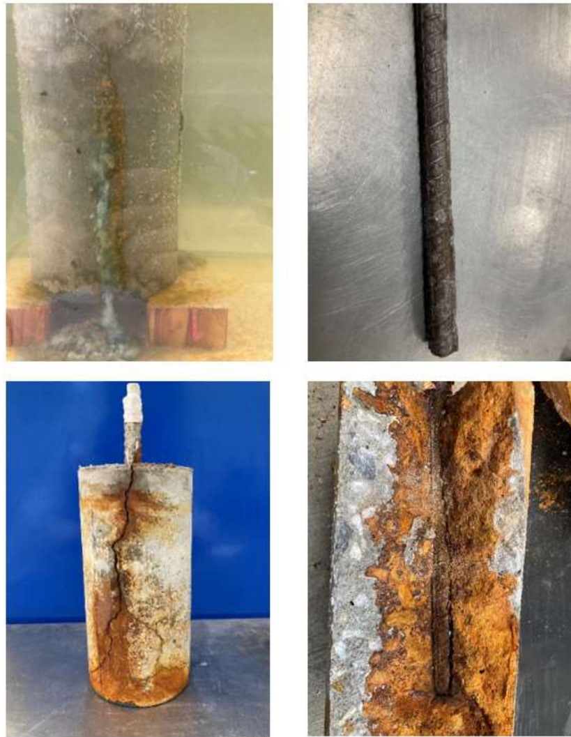
Figure 4-13 (Top left) ACIC specimen during the test with corrosion byproducts oozing out, (Bottom Left) Cleaned cracked specimen with crack pattern parallel to the embedded N12 rebar, (Top right) Extracted corroded N12 rebar with heavy corrosion and pitting signs, (Bottom right) Corroded specimen cut parallel to the central axis to extract rebar, the corrosion by-products can be seen on the surface of the concrete by brown, dark brown and black colours
