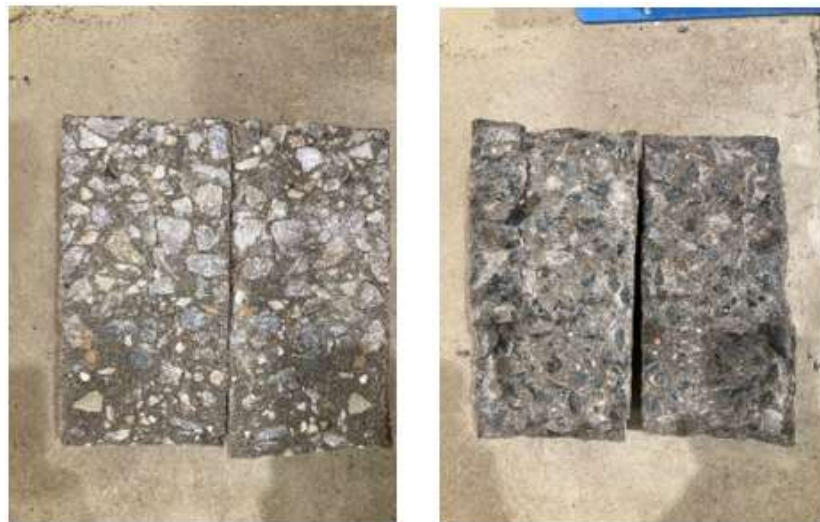
Figure 4-5 (left) Non-reactive specimen undergone indirect splitting tensile strength test (Right) Reactive specimens undergone indirect tensile strength test
