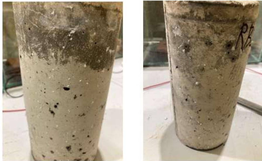
Figure 4-14 Reactive cylindrical ( \varnothing 100\text{mm} \times 200\text{mm} ) specimens with an N12 steel reinforcement with ASR gel exuding and microcracking on the surface
