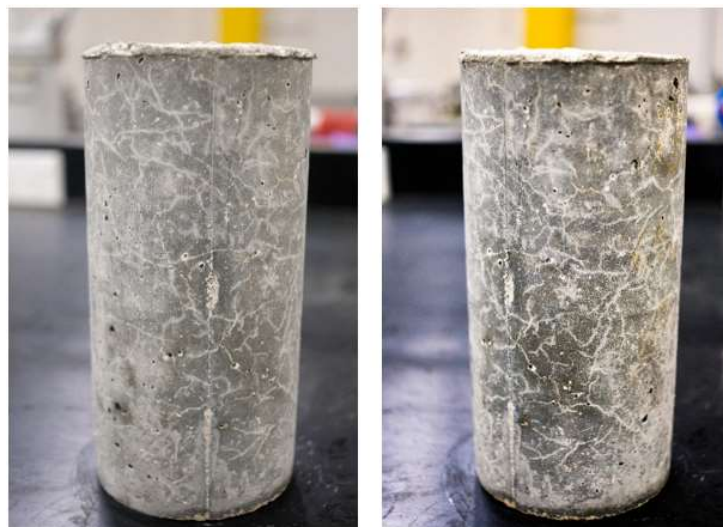
Figure 4-3 External cracks on cylinders after 120-days submerged in 1M sodium hydroxide solution in 38°C climate chamber
