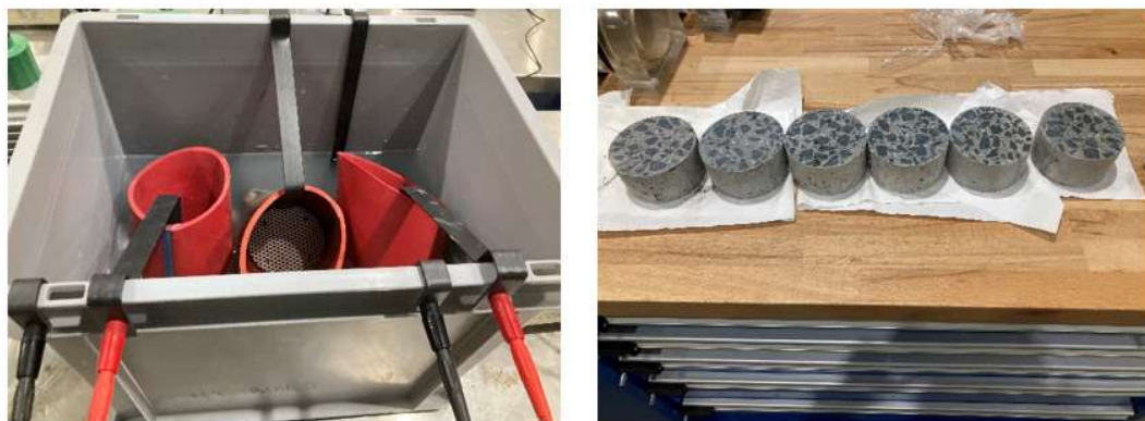
Figure 4-23 (Left) NT build 492 test tank and (Right) Specimens ready for NT build 492 test after extracting from the vacuum chamber
