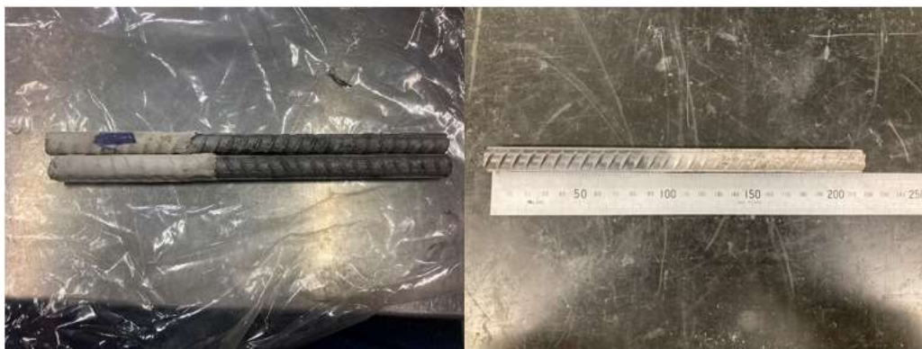
Figure 4-21 (Left) Extracted unclean corroded rebars, (Right) Sandblasted rebar the left side of the rebar, which was covered in epoxy, has no signs of corrosion, while the right side is heavily corroded with signs of pitting corrosion
