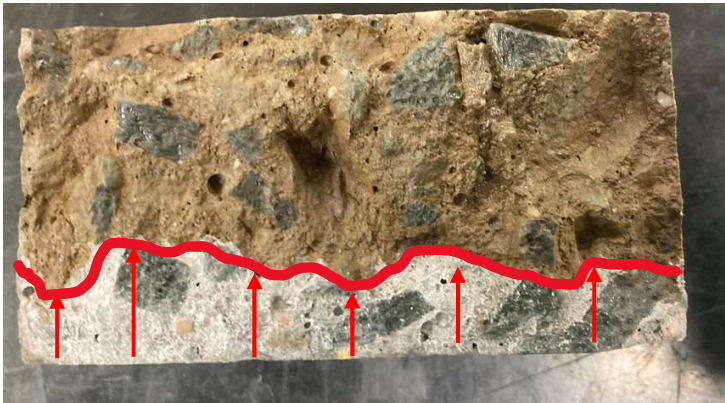
Figure 3-18 Chloride precipitation and direction of penetration
