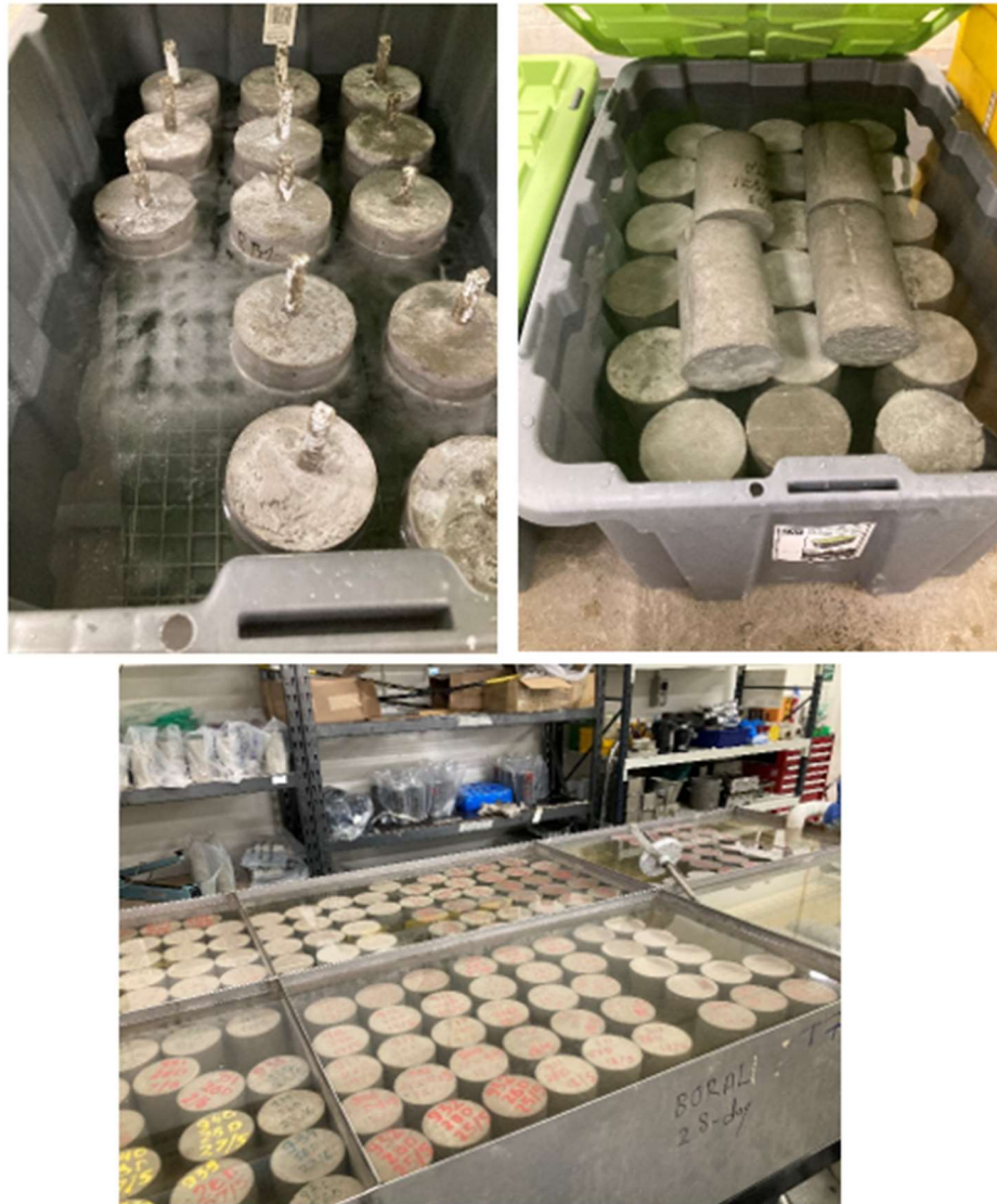
Figure 3-11 (Top) Reactive and non-reactive specimens in 38°C climate chamber with non-reactive specimens being submerged in water and reactive specimens submerged in 1 M sodium hydroxide (NaOH) solution, (Bottom) Non-reactive and reactive specimens cured in 25°C submerged in water.
