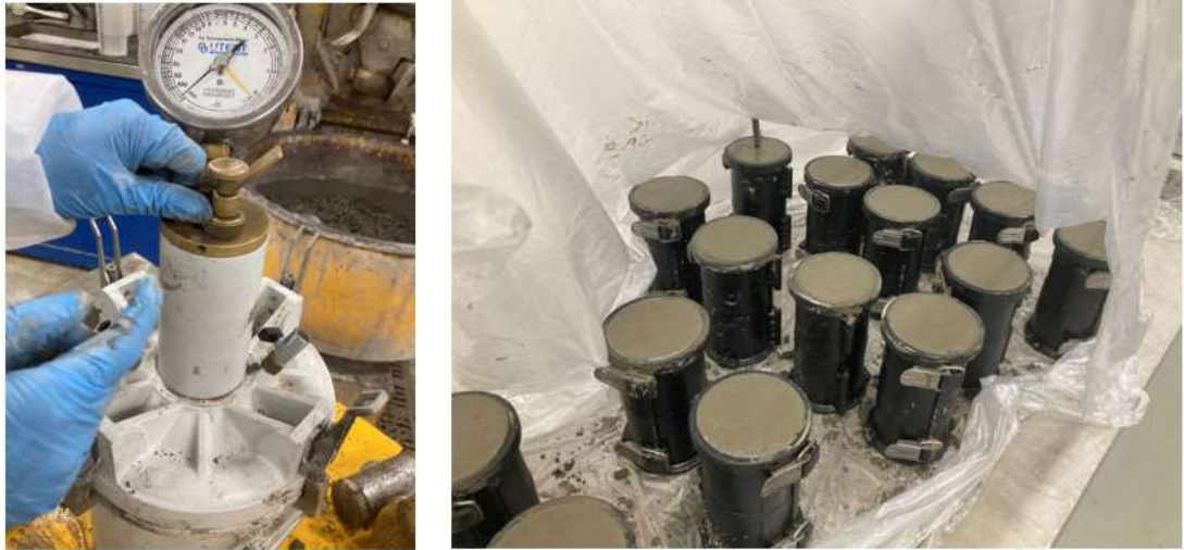
Figure 3-10 Pictures of concrete mixing process with slump, air content and density test measurements at UTS Tech Lab
