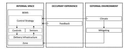
**Figure 1.** The schema representation of a typical BEMS
