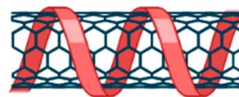
Figure 7. Structural representation of a carbon nanotube.
