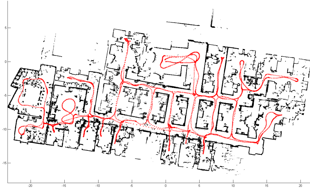
Figure 3: Pose-Only SLAM Map of CAS
