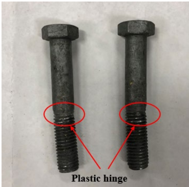
Fig. 12. Failure modes of the specimens with M12 nut and bolts: (a) crushing of plywood; (b) bolt head bearing into plywood; (c) plastic hinge
