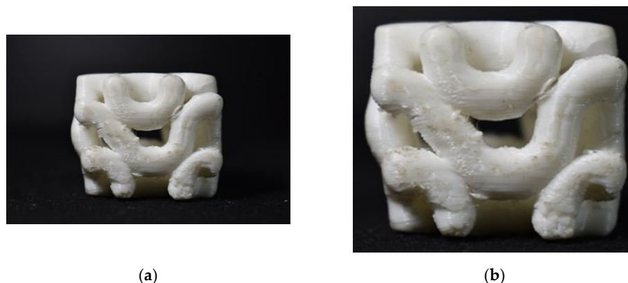
Figure 19. (a) A 3D printed AGM; (b) Tested model with failed structure.
