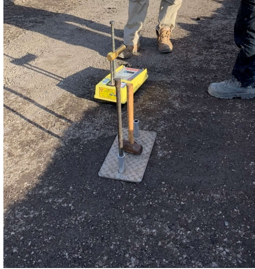
Figure 8.6 Non-destructive density testing for the capping layer
