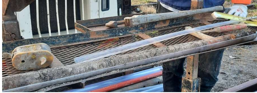
Figure 8.1 Soil sampling refusal at proposed RIBS section of track
