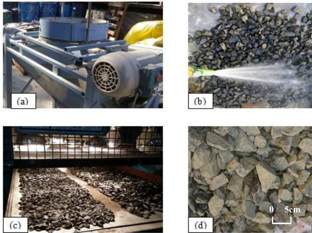
Figure 3.5 Ballast material preparation (a) vibrating shaker, (b) washing, (c) drying, and (d) prepared ballast
