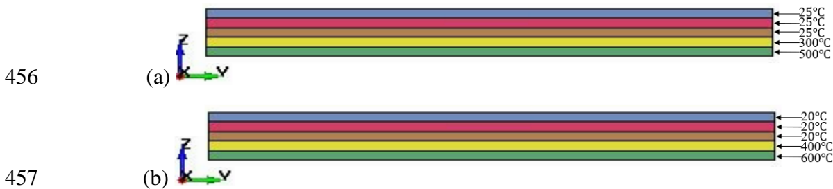
458 Figure 12. Temperature distribution for RC slab with 2 hrs fire-exposed time. (a) NSC (b) 459 UHPC
