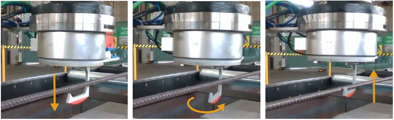
Figure 2: The gripper is a tine that hooks under a bar and lifts it. The tine moves down next to the bar being lifted (left), rotates beneath the bar (middle), and then lifts to softly engage the bar(right).
