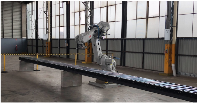
Figure 5: The ABB IRB6700-200/2.60 robot, located at the ARM Hub along with the experimental conveyor.
