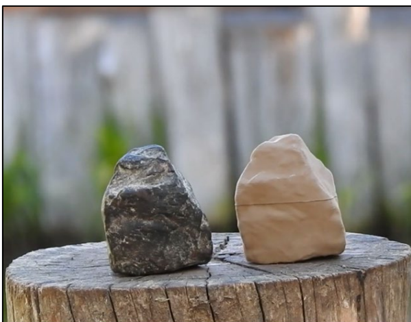
Figure 54: Smart Ballast particle (unpublished part of a current program at the University of Technology, Sydney through funding from the Australian Research Council), courtesy A. Siddiqui, PhD student)
