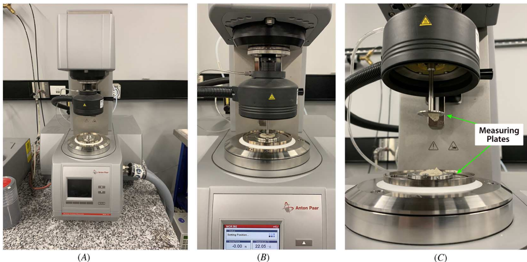
FIG. 3 (A) Rheometer (MCR302) test setup used in this study. (B) The sample is placed in the bottom measuring plate while the top measuring plate is lowered, (C) and the top measuring plate is raised after the test.
