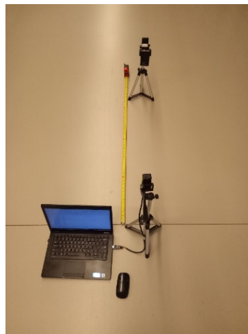
Figure 4. Testbed setup for 1-m distance range for UWB localization.
