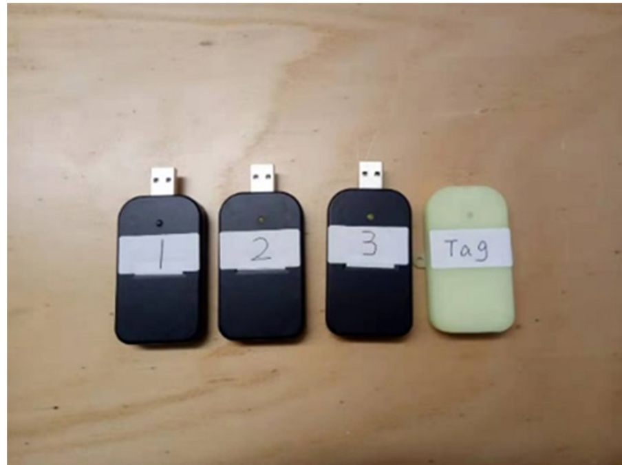
Figure 2. Three UWB Anchors and one UWB tag.
