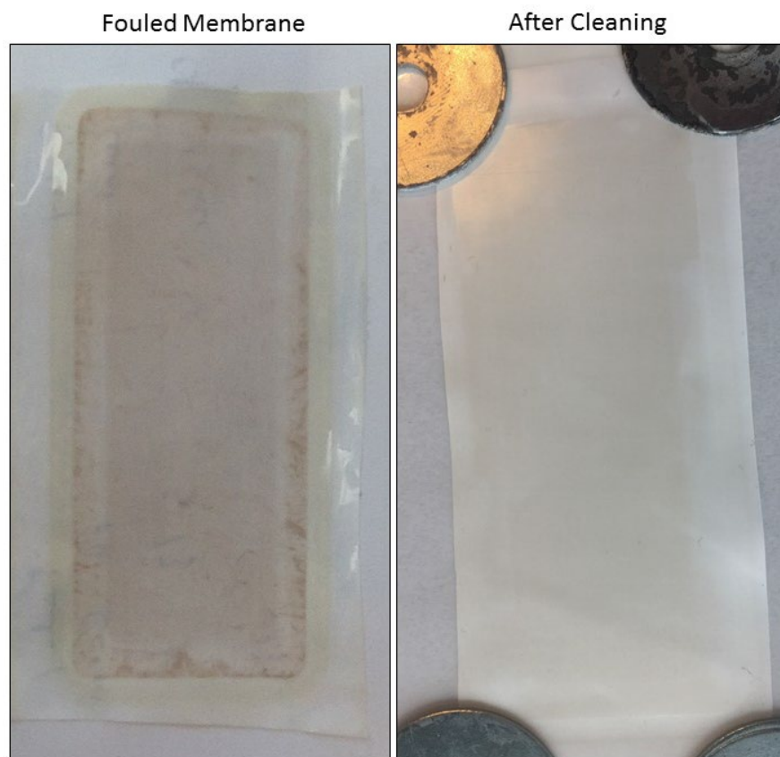
Figure 6-4 Picture of the membrane coupon before and after the alkaline cleaning. The feed solution was real urine while the draw was commercial fertiliser. The experimental run time was 11 days.
