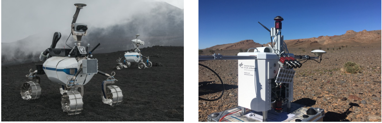
Figure 2: Pictures of the Lightweight Rover Unit (LRU) rovers on Mt. Etna (left) and the Sensor Unit for Planetary Exploration Rovers (SUPER) handheld system in the Morocco desert (right).
