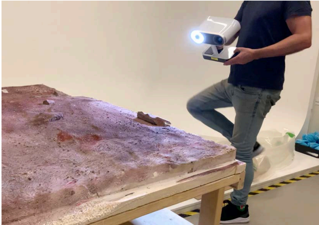
Figure 5.8: Artec Leo scanning a temporary test miniature set.
