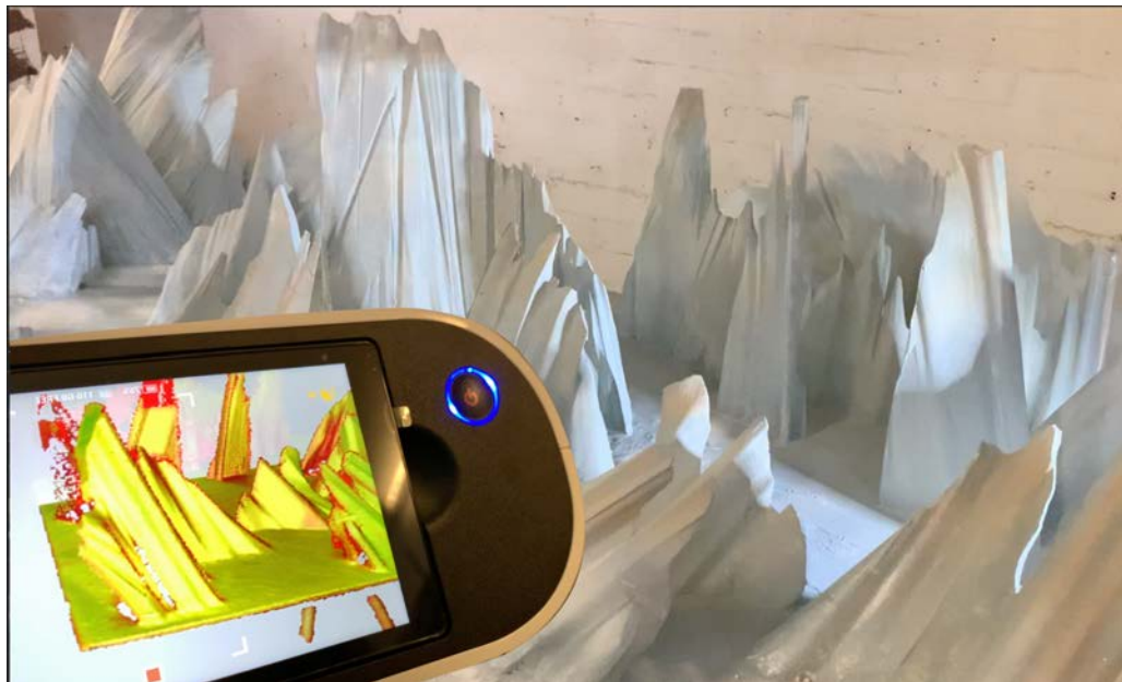
Figure 5.29: Moon surface miniature set being scanned.
