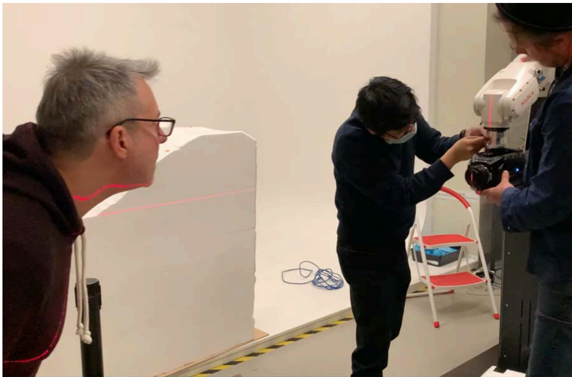
Figure 5.12: VFX artist Andres Wanda and the research team using a laser tool to align the camera and robot set-up.
