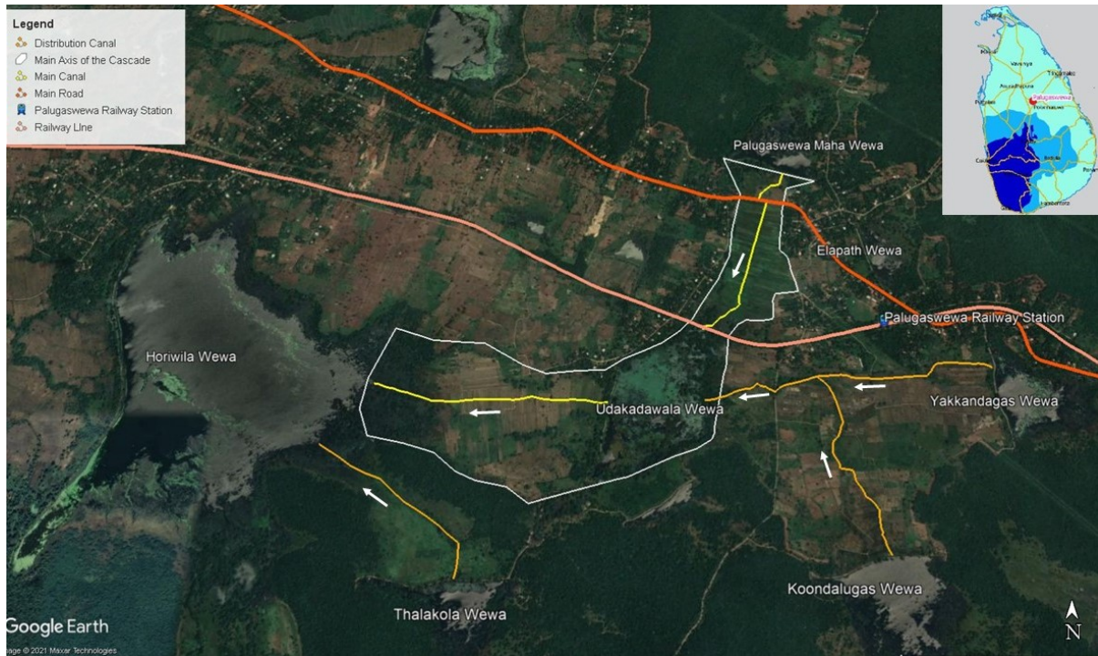
Figure 14 - Palugaswewa Tank Cascade System, white polygon shows the main axis of the cascade, yellow lines show main “canal” moving spillover on the main valley of the cascade, orange lines shows “canals” moving spillover from tanks in the side valleys into the main valley, white arrows indicate the direction of water flow.
