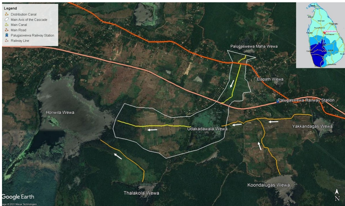
Figure 10 - Palugaswewa Tank Cascade System (White polygon shows the main axis of the cascade, yellow lines show main “canal” moving spillover on the main valley of the cascade, orange lines show “canals” moving spillover from tanks in the side valleys into the main valley, white arrows indicate the direction of water flow.
