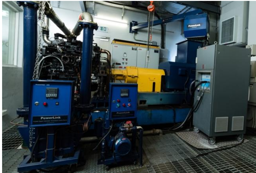
Figure 2: Heavy-duty transient engine dynamometer test cell with a Euro V diesel bus engine in Hong Kong Jockey Club Heavy Vehicle Emissions Testing and Research Centre (JCEC).
