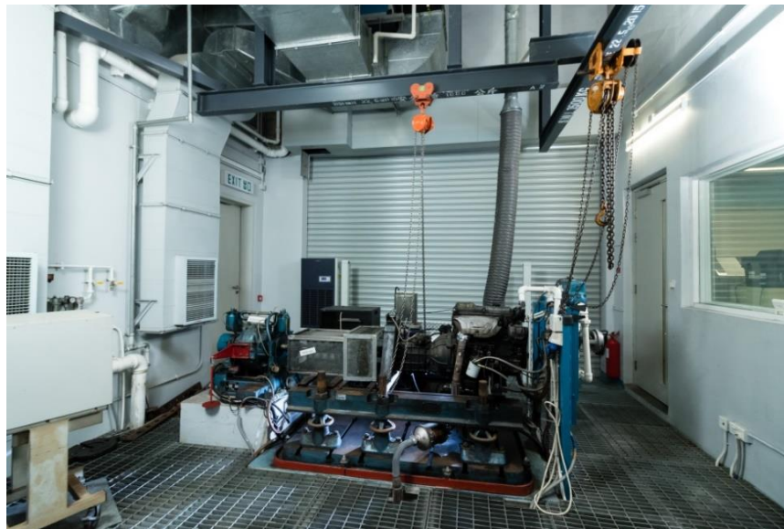
Figure 3: Light-duty eddy current engine dynamometer test cell with a Euro 3 diesel engine in Hong Kong JCEC.
