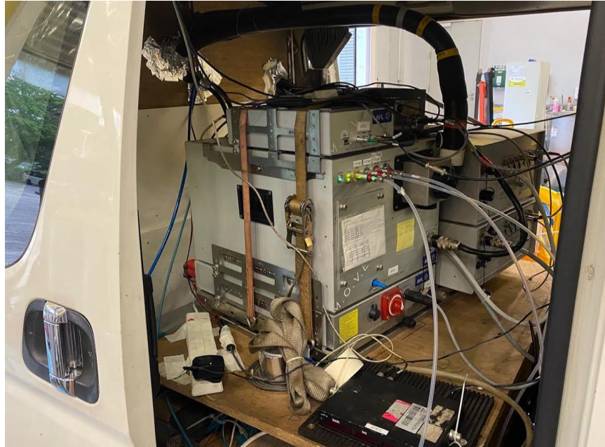
Figure 20: AVL gas PEMS installed on the test vehicle.
