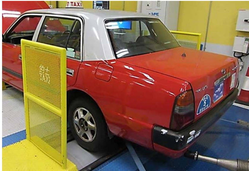
Figure 4: Light-duty transient chassis dynamometer in Hong Kong JCEC.
