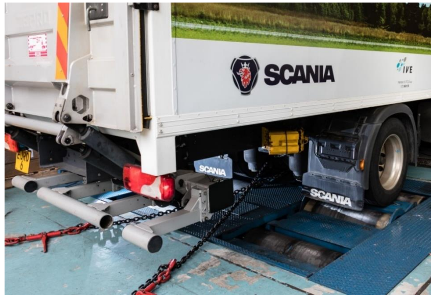
Figure 5: Heavy-duty transient chassis dynamometer in Hong Kong JCEC.
