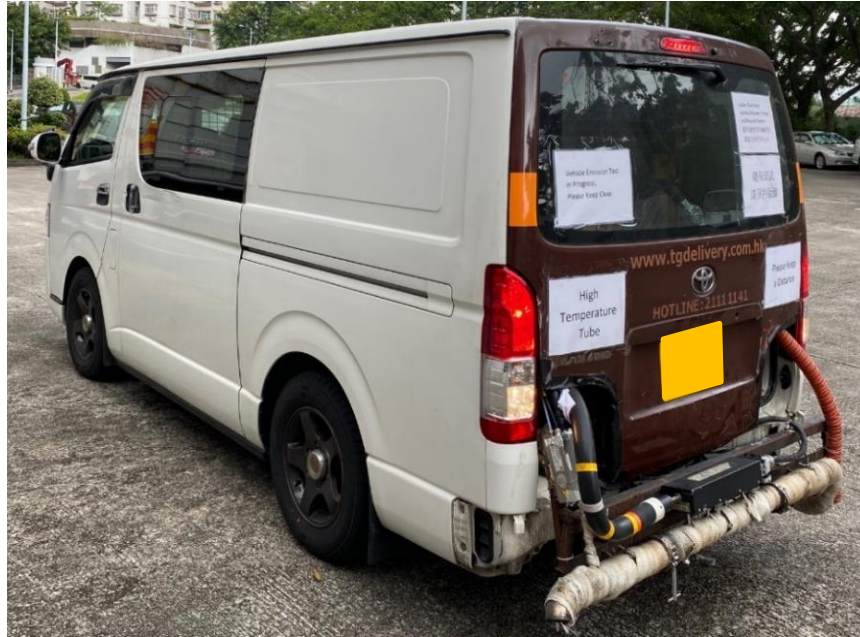
Figure 22: Test vehicle exhaust connected with the emissions gas sample line and exhaust flow measurement system.
