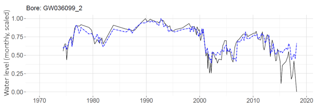
Figure 15. Prediction on an untelemetered well using global MLP (blue, dashed) over measured data (black). RMSE = 0.195.
