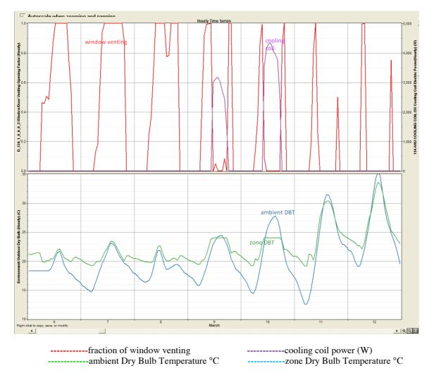
Figure 1: Mixed mode prediction using EnergyPlus
