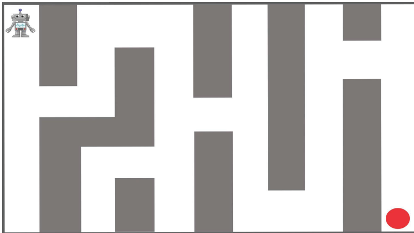
Fig. 4 A simple example of reinforcement learning, in which a robot tries to find an object in the Grid World environment. The blue robot can be seen as the agent in reinforcement learning. The red circle is the target object. The grey boxes denote the obstacles, while the white boxes denote the road. The robot’s purpose is to find a route to the red circle.
