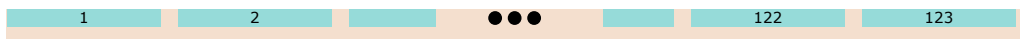
(c) A repetition code made up of surface code patches, with 123 surface patches as in Fig 17b, p_x < 1.39 \times 10^{-16} , p_Z < 2.10 \times 10^{-16} .
