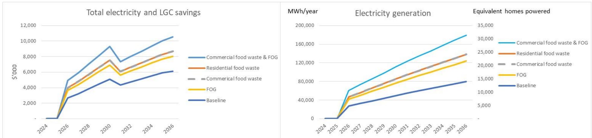
Figure 11: Electricity generated from biogas in MWh/year for the different scenarios, with the equivalent number of homes powered, and the value of the electricity.
