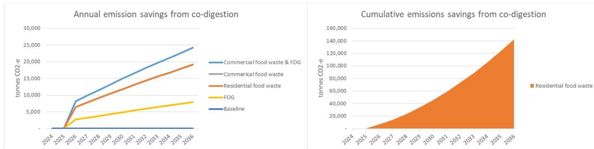
Figure 13 Annual greenhouse gas emission reduction by scenario and cumulative emission savings for residential food waste (co-digestion at AWRC)
