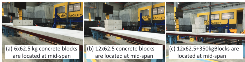
Fig. 5. (a) first load case - 375kg, (b) second load case - 750kg, and (c) third load case - 1100kg.
