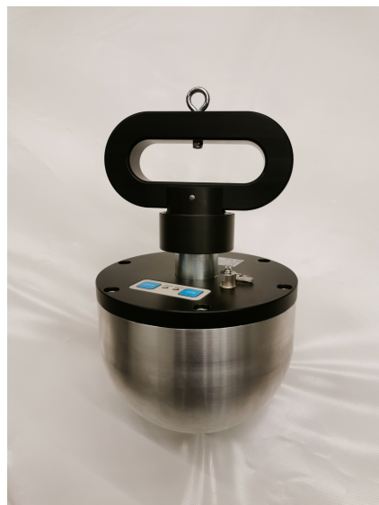
Figure 8. The HIC impact test meter used in this research.
