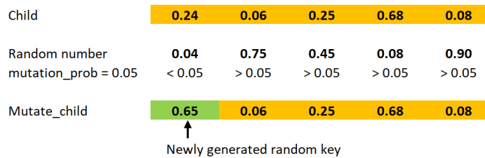
Figure 3.4: Mutation example. For each gene, one random number is generated from U(0, 1) . Since the random number of gene 1 is smaller than mutation\_prob (i.e., 0.04 < 0.05 ), the corresponding gene value is replaced by a new random key, i.e. 0.65.
