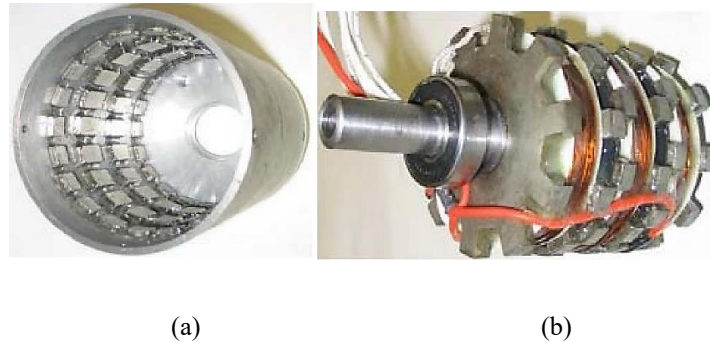
Fig. 4-4. Prototype of the PM TFMSM: (a) Rotor, (b) Stator.
